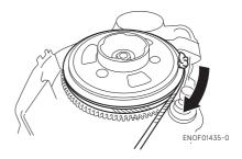
5. Tie a loop in the another end of the emergency starter rope and attach socket wrench, Both the loop and the wrench are provided in outboard motor box.
