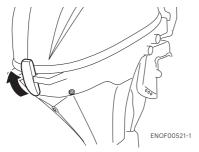
2. Remove starter lock cable from recoil starter by loosening the screw for the starter lock cable.
