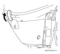
2. Remove starter lock cable from recoil starter by loosening the screw for the starter lock cable.
