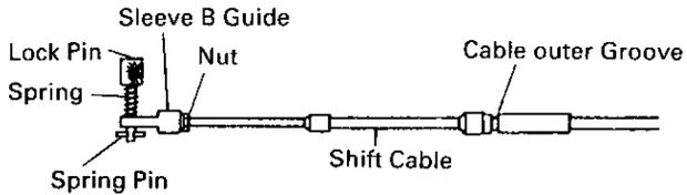
② Fitting of Remote Control Cable to Engine
