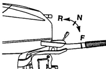
Be sure that the shift is in neutral when starting the engine.
